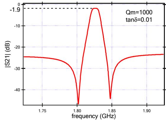
Figure 9. Frequency response of an optimized filter.
