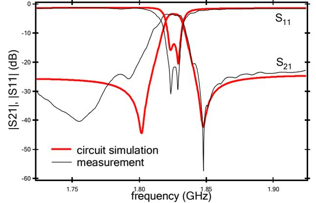
Figure 7. Equivalent circuit simulation fitted to the measurement.
