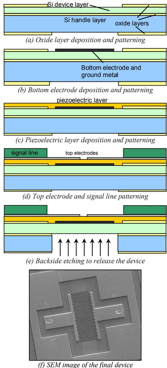
Figure 4. The abbreviated process flow of the TPoS filter.
