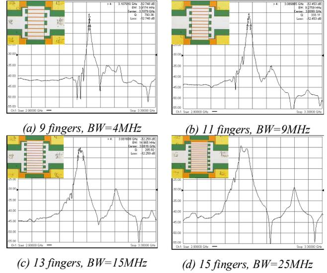
Figure 6. Bandwidth tuning measurement of TPoS filters with different finger numbers
