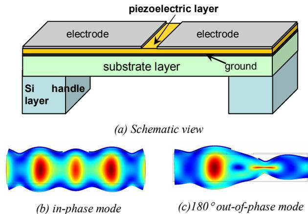
Figure 1. The schematic view and the resonance mode shapes of a thickness-mode TPoS filter.
