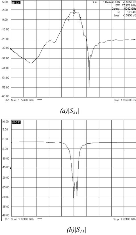
Figure 5. The measured  $|S_{21}|$  and  $|S_{11}|$  plots of a TPoS filter (with 50Ω termination).
