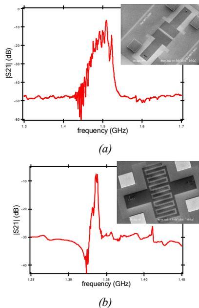
Figure 3. Typical frequency response of filters with (a) two simple rectangular electrodes and (b) IDT electrodes.
