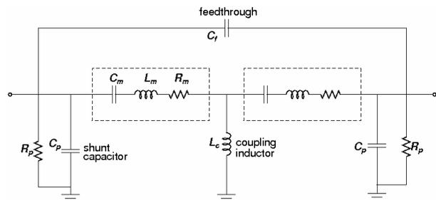
Figure 2. The equivalent circuit of a TPoS filter.
