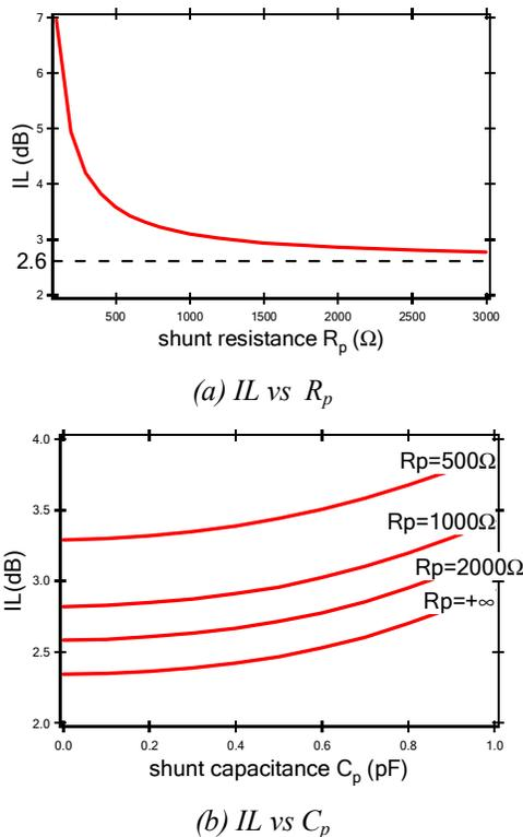
Figure 8. The relationship between IL and (a) the shunt resistance  $R_p$ , (b) the shunt capacitance  $C_p$ .
