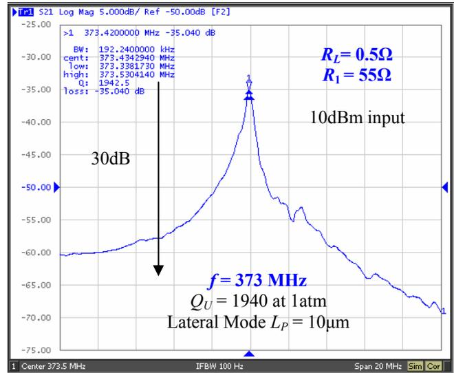
Figure 8: Freq. response of a 9<sup>th</sup> mode resonator with  $L_P=10\mu\text{m}$  at 1atm
