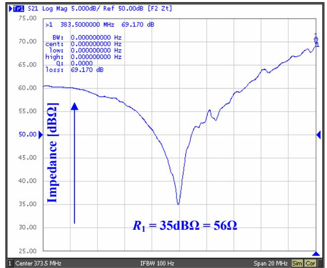
Figure 9: Impedance of a 9<sup>th</sup> mode resonator with  $L_P=10\mu\text{m}$  at 1atm [dBΩ]
