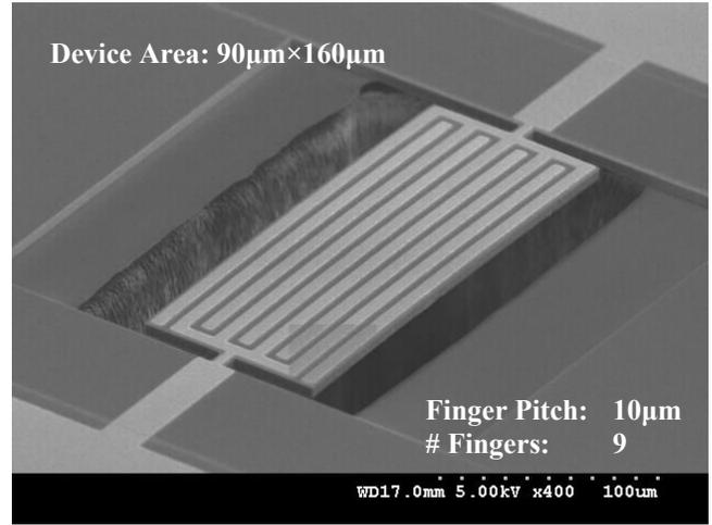
Figure 7: SEM of a 90µm×160µm CBAR with  $L_P=10\mu\text{m}$
