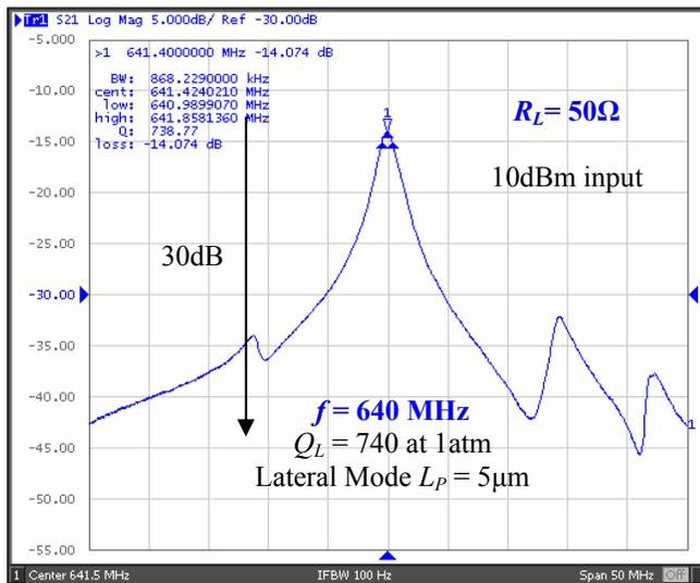
Figure 10: Frequency response of a 15th mode resonator with  $L_p=5\mu\text{m}$  at 1atm
