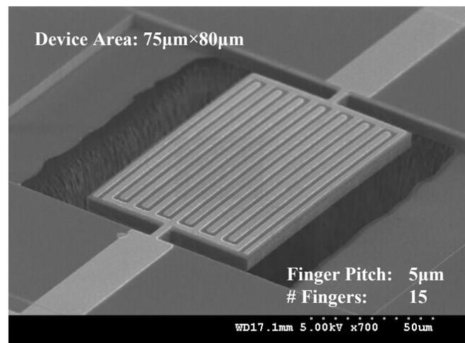
Figure 2: SEM of a 640MHz CBAR ( $L=75\mu\text{m}$ ,  $w=80\mu\text{m}$ )
