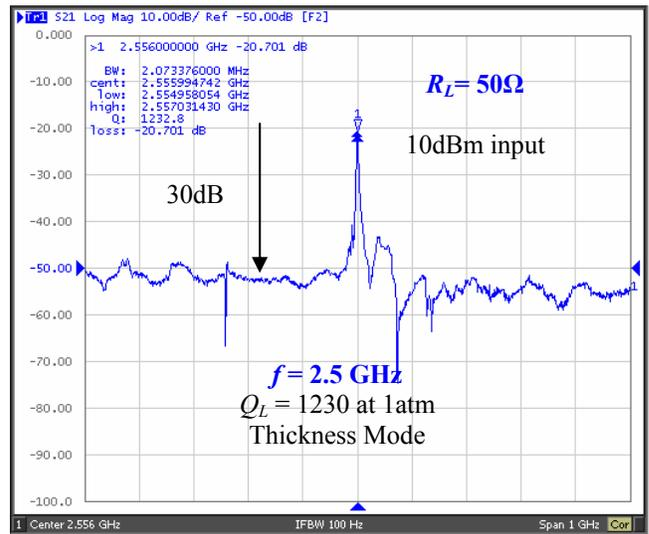
Figure 11: Frequency response of a thickness mode resonator fabricated on the same substrate as the CBARs
