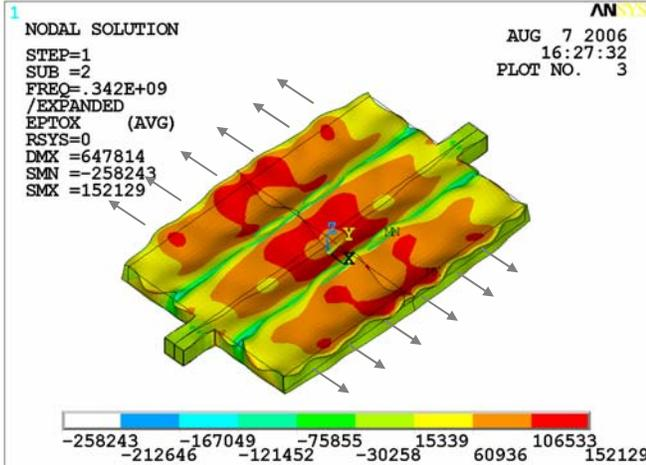
Figure 6: Simulated mode shape of a fifth-order ZnO-on-SCS CBAR with a finger pitch of 10µm
