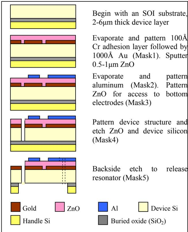
Figure 3: Fabrication process flow for ZnO CBARs
