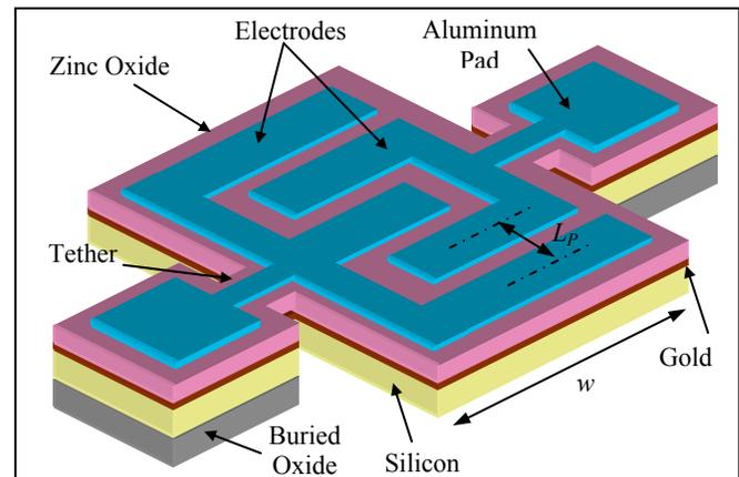
Figure 1: Composite piezoelectric-on-silicon micro-mechanical bulk acoustic resonator
