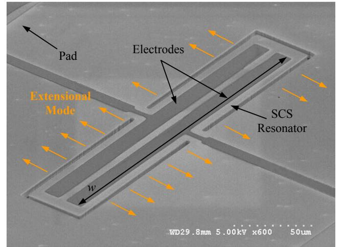
Figure 4: SEM of a 240µm×40µm fundamental-mode CBAR
