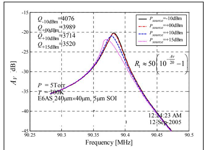
Figure 5: Linearity of a fundamental width-mode CBAR,  $Q=4000$ .  $P_{1dB} = 10dBm$ .
