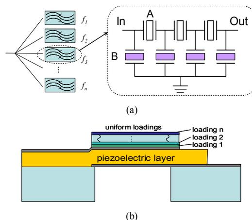
Figure 1. (a) System and filter architecture and (b) schematics of a single resonator for ladder-type FBAR filter based multi-channel systems.
