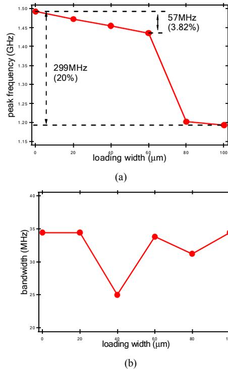
Figure 7. (a) Peak frequency and (b) 3dB bandwidth vs. loading layer's width in the filter array.
