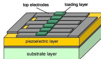
Figure 4. The schematic view of a TPoS filter with interdigitated top electrode and loading layers.
