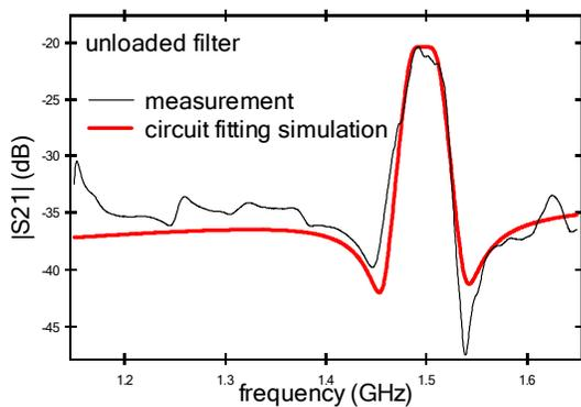
Figure 9. Equivalent circuit simulation fitted to the measurement data.
