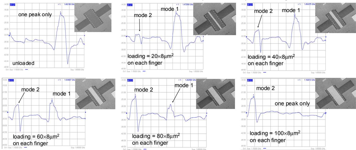
Figure 6. Measured frequency response of an array of filters with different loading width ( $50\Omega$  termination).
