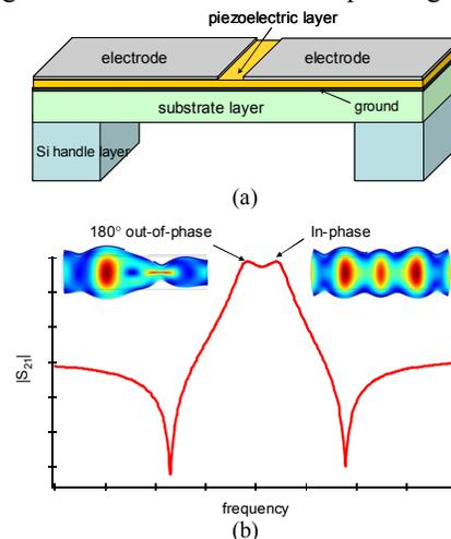
Figure 2. (a) The schematic view and (b) mode shape illustration and simulated frequency response of a thickness-mode TPoS filter.
