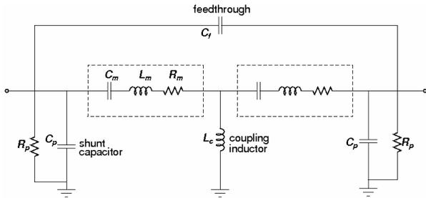
Figure 8. The equivalent circuit of a TPoS filter.
