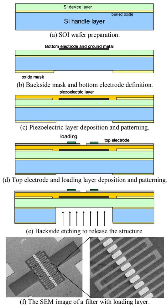
Figure 5. The abbreviated process flow and the SEM image of a loaded filter.
