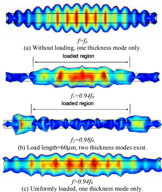
Figure 3. Simulated resonance mode shapes of a  $100\times 5\mu\text{m}^2$  ZnO film loaded by a thin Au layer of 100nm thickness and variable width.
