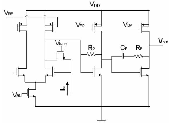
Fig. 3. Schematic diagram of the TIA (biasing not shown)
