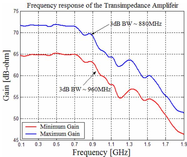
Fig. 4. Frequency response of the tunable TIA
