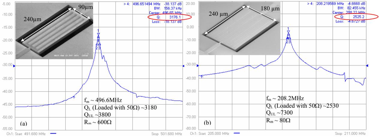
Fig. 2. SEM view and frequency response of (a) 496MHz, (b) 208MHz AlN-on-Si resonators
