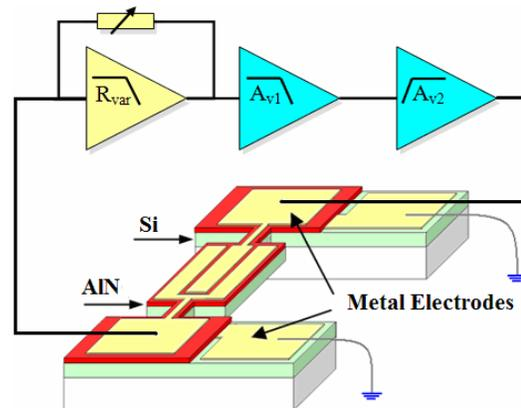
Fig. 1. Block diagram of the piezoelectric oscillator.
