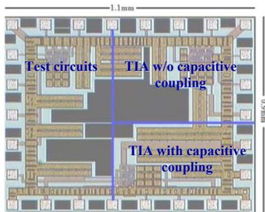
Fig. 5. Micrograph of the fabricated die
