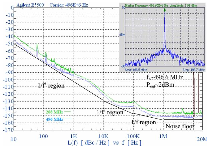
Fig. 6. Measured phase-noise of 496MHz and 208MHz oscillators. The spectrum of output waveform for 496MHz is also shown.
